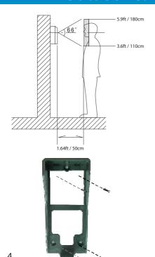
To mount the outdoor camera run the cable from the Doorphone and pull it through the hole you created at the camera mounting point, and then use the four screws to secure the mounting bracket to the wall with the wire inside the bracket so you can connect the camera.
